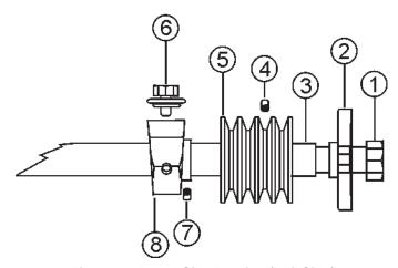
Figure 51. Pulley Side Bearing (Left Side)
